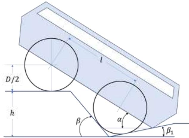
The mathematical model of the rover indicates that the maximum angle  $\alpha$  it can traverse, given the maximum angle  $\beta$  at which its underside remains clear of the ground, satisfies the following equation:
